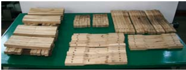
Fig. 5. Sets of the specimens for tensile, compressive and flexural tests after testing
