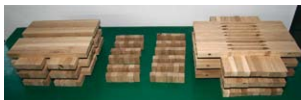
Fig. 4. Sets of the specimens for tensile, compressive and flexural tests before testing
