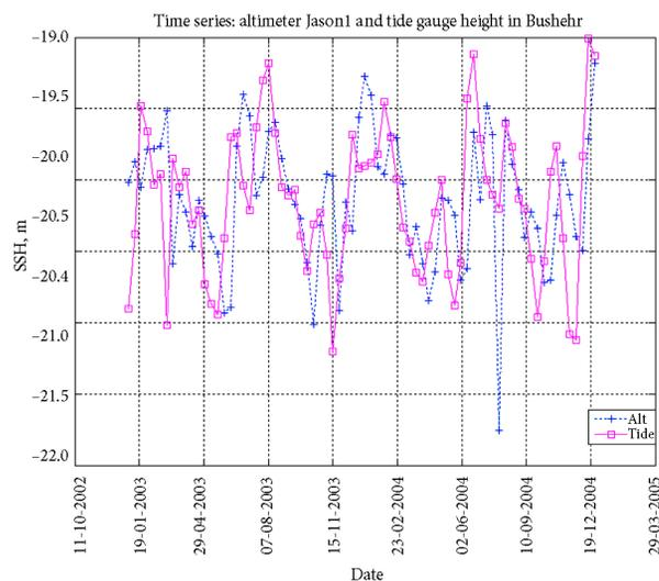
Fig. 6. SSH time series obtained from Jason-1 versus those of Bushehr tide gauge over a 2-year time span from 2003 to 2005
