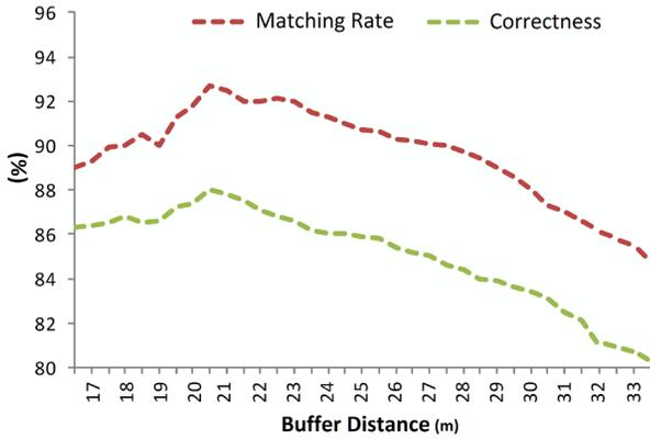
Fig. 19. Sensitivity analysis for the buffer distance
