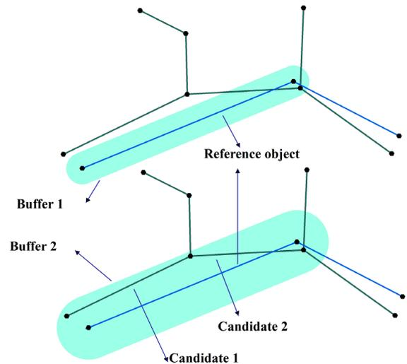
Fig. 9. Buffer expanding in the width direction
