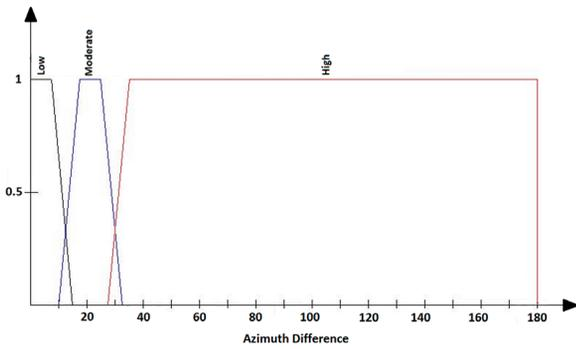
Fig. 11. Membership functions of azimuth difference
