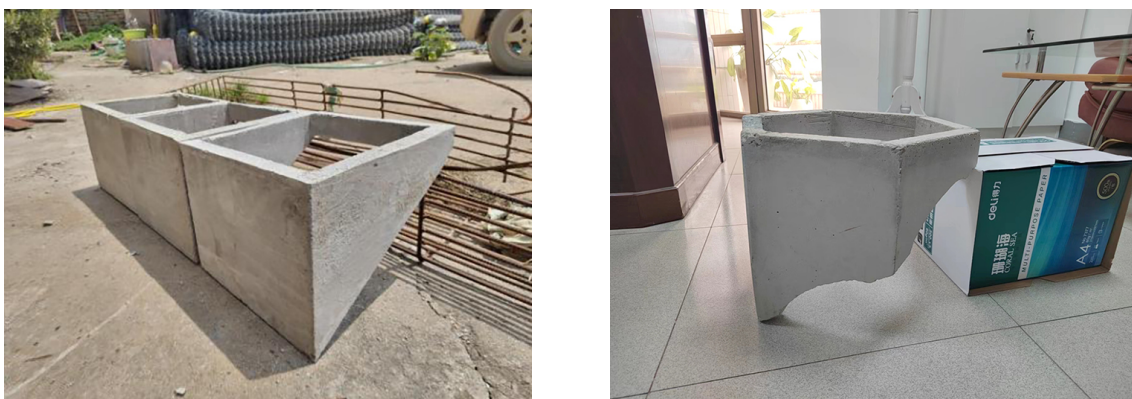
Figure 6. Samples of finished recycled concrete structural member
