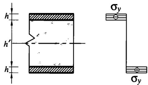
Fig 4. Three-layered bending plate cross-section
