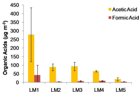
Fig. 5. Organic acids (acetic and formic acids) concentration measured in the LTMCM. Values represent the average from two parallel samplers. For abbreviations and location characteristics see Table 1
