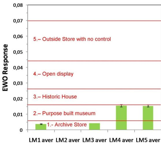
Fig. 2. EWO dosimeter responses (ΔLight absorbance) obtained in the five indoor locations in the LTMCM
