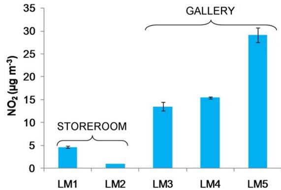
Fig. 3. NO<sub>2</sub> concentration obtained in the LTMCM. Values represent the average from two parallel samplers. For abbreviation and locations characteristics see Table 1
