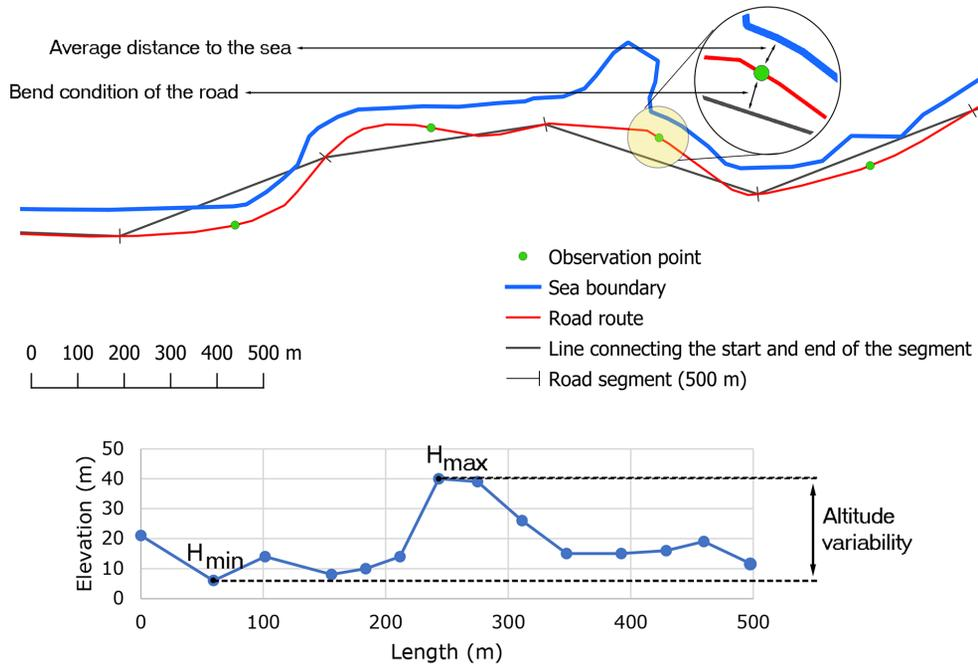
Figure 2. Measurement method of road properties
