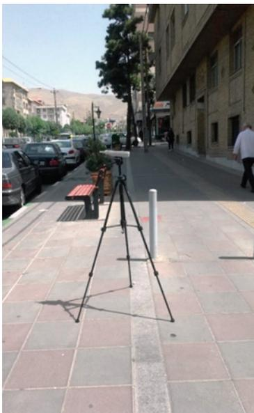
Figure 2. Placement of sound level meter on sidewalk to measure traffic noise
